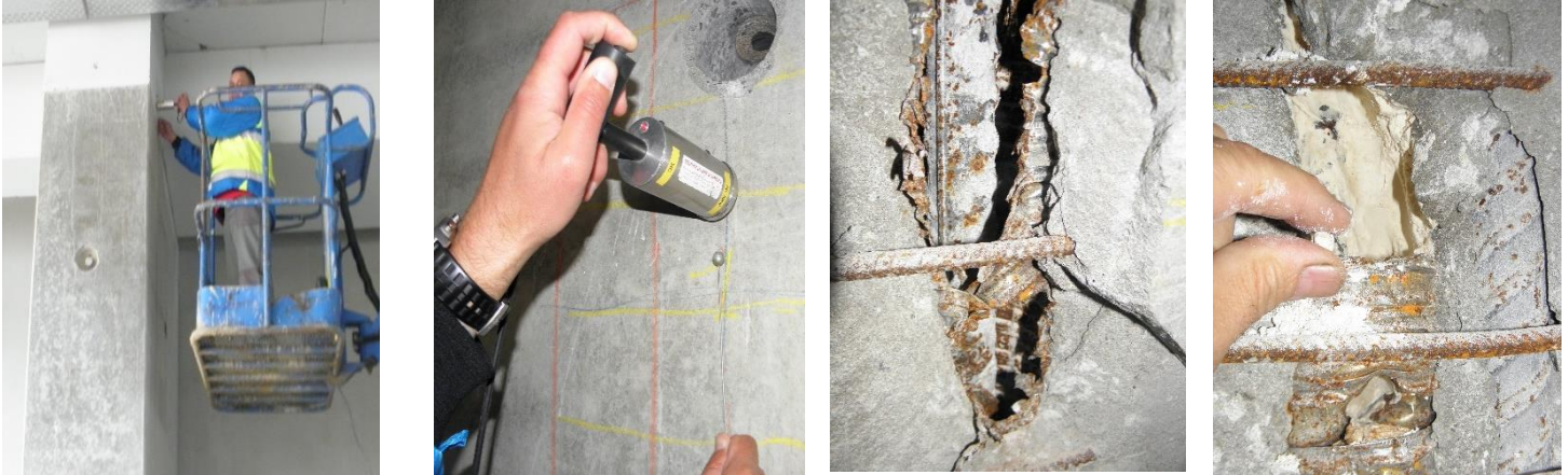
Implementation of DOCTer Impact-Echo for detection of voids in cable ducts, Belgium
