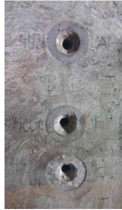
Implementation of CAPO-test for testing of columns to be further loaded, Houston, USA
