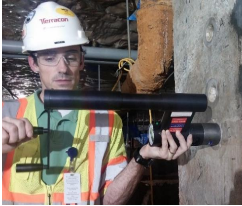
Implementation of CAPO-test for testing of columns to be further loaded, Houston, USA
