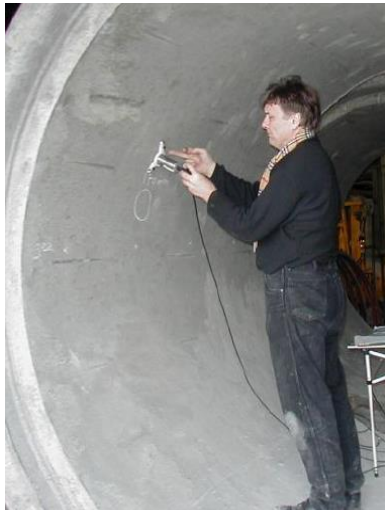
Implementation of DOCTer Impact-Echo for detection of voids in cable ducts, Belgium
