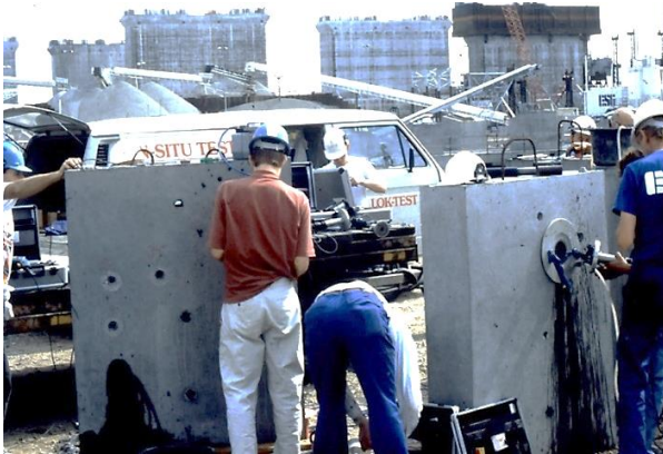
Training course at the Danish Great Belt Link in LOK-test and CAPO-test for production control of the GBL structures
