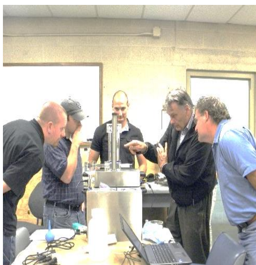
Implementation of AVA for air void structure of fresh concrete, FHWA, Topeka, Kansas, USA
