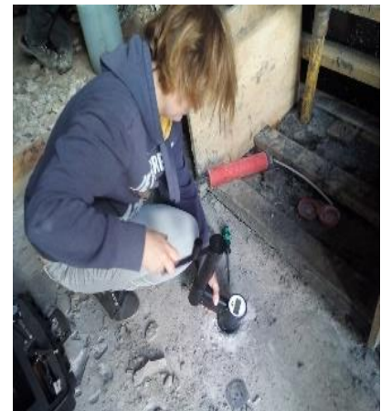
Implementation of CAPO-test on joints before loading of a bridge deck, Kentucky, USA
