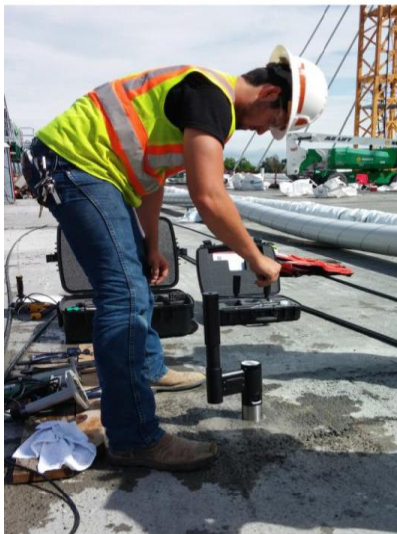
Implementation of CAPO-test on joints before loading of a bridge deck, Kentucky, USA
