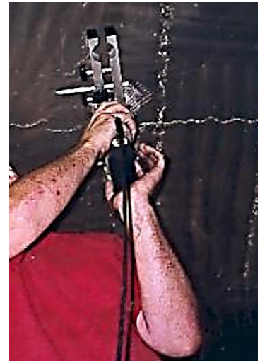
Implementation of DOCTer Impact-Echo for detection of voids in cable ducts, Belgium
