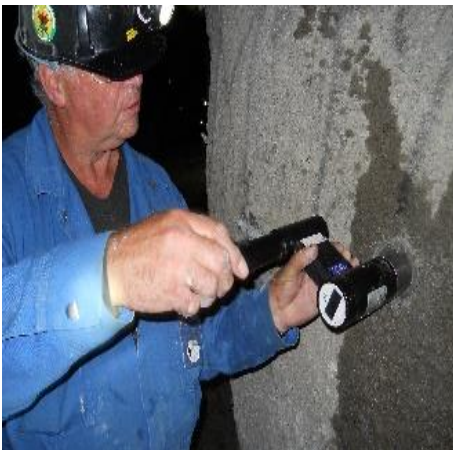
Implementation of CAPO-test on joints before loading of a bridge deck, Kentucky, USA
