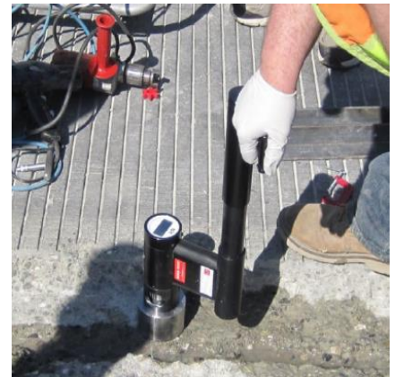
Joint testing at Anchorage Airport runway, Alaska Testing of substrate before applying the joint overlay
