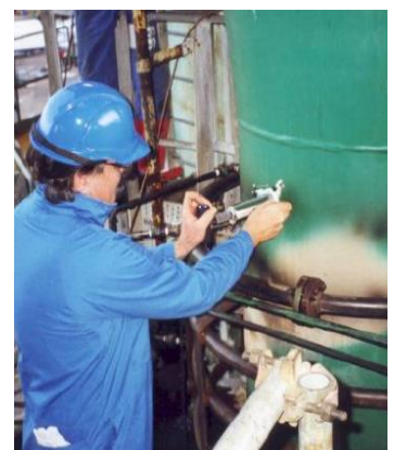
Thickness of concrete liner inside riser column, Sweden
