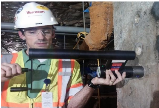
Columns, Houston Strength before further loading
