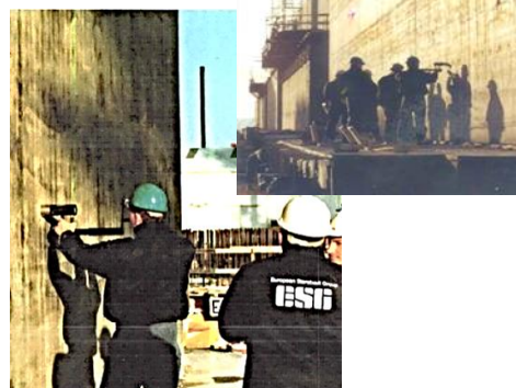
CAPO-testing on the Caissons of the GBL West Bridge
