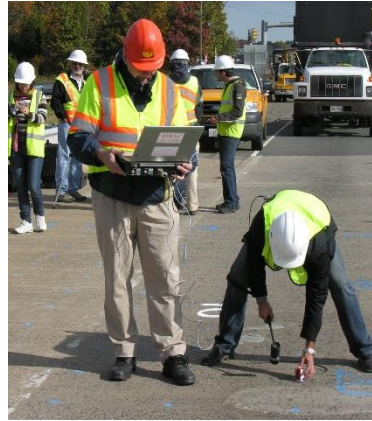
Bridge Slab, Virginia Voids / lack of support
