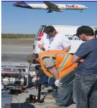
Joint testing at Anchorage Airport runway, Alaska Testing of substrate before applying the joint overlay
