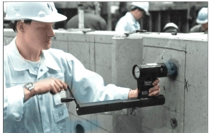
Certified CAPO-TEST technician Henrik Kristensen performing the CAPO-TEST on the tunnel elements.
