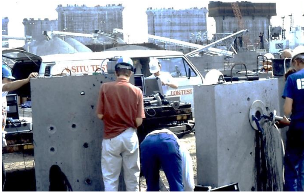
Great Belt Link, Denmark LOK-TEST and CAPO-TEST training for production control with emphasis on the cover layer
