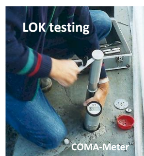
Coma-Meter, maturity is registered automatically, to the left showing 1.3 M 20 days, obtained after 0.5 actual day
