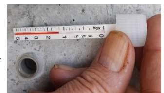
Coma-Meter, maturity is registered automatically, to the left showing 1.3 M 20 days, obtained after 0.5 actual day
