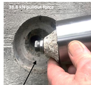
38.8 kN pullout force testing surface 32 mm deep
