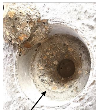
testing surface 30 mm deep, pullout force 30.0 kN compared to 29.5 kN 25 mm deep
