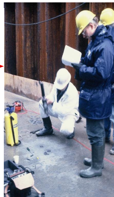
The six CAPO-test performed, all with acceptable failures, cf ref 2, page 24.
