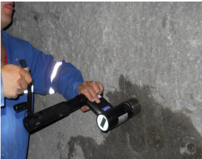
The hydraulic CAPO-TEST instrument is coupled to the coupling and the slack removed between instrument and counter pressure. Loading takes place by turning the instruments handle slowly.
