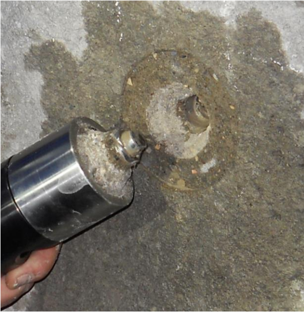
The completed CAPO-TEST. Notice the unfolded CAPO ring on the cone pull bolt. And, the failure surface is not affected by water intrusion from the water used by coring or planning
