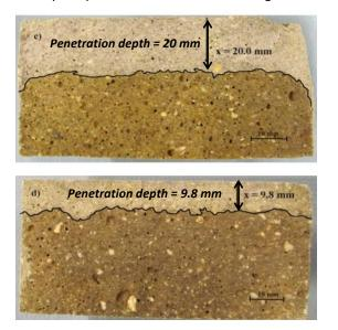
chloride ions into the concrete specimen so that their depth of penetration can be measured.
