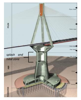
critical exposure zone, the splash and tidal zone, identified as the zone between -5 m and +10 m from the medium see level,
