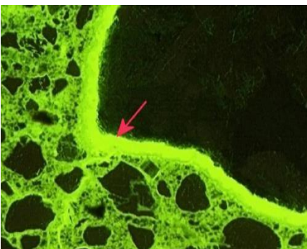
5. Thin section, 1 mm x 1.5 mm, from concrete suffering from DEF, Delayed Ettringite Formation. Severe internal expansion may occur if the concrete had high temperature at casting/early curing. This can happen years after casting when moisture becomes available.
