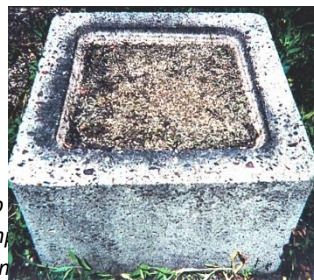
Example 2 of outdoor exposure to Freezing and Thawing after 40 years. Left: Concrete with improper air-void system. Right: concrete with correct air entrainment.
