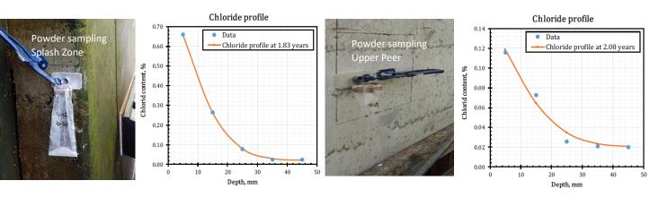
In 2013 the construction began of the new 47,000 square meter container terminal in Nuuk, Greenland, and was opened to operation in 2017. Some months later, under suspicions of low strength concrete in some elements of the peers, investigations of chloride penetration in the cover layer were carried out using the Germann Instruments' RCT (Rapid Chloride Test).
