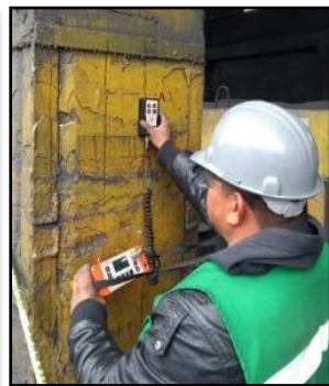
Covermeter for size of bar
