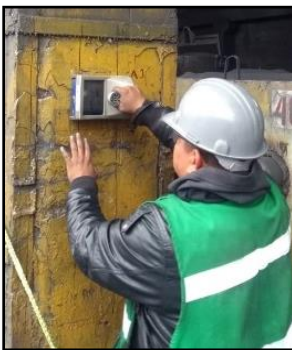
GPR for rebar depth
