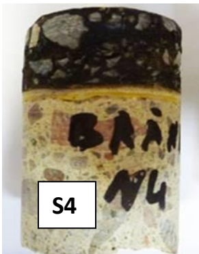
Green areas have the lowest mobility (sound), the yellow higher and the red the highest mobility (not sound) For calibration to the mobility, BOND-TEST's were made at test poinr S4 and S3, examples below.
