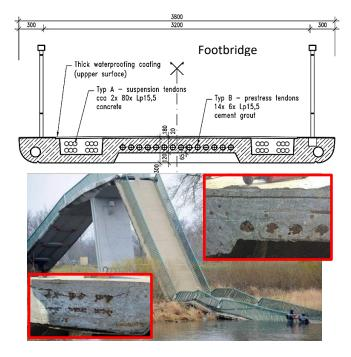
After the collapse of the Troja stressed ribbon concrete footbridge in Prague, Czech Republic, due to corrosion of the prestress steel strands, **NDTitans Claus Petersen**, **Malcolm Lim and Hugo Orozco** were invited to demonstrate the feasibility of utilizing different nondestructive testing techniques to evaluate the current condition of similar stress ribbon bridges located in the country.
