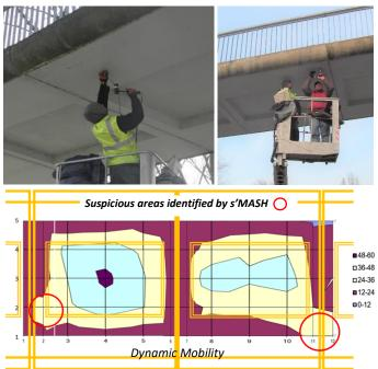
A preliminary visual inspection found moisture stains on the underside of the bridge caused by the water leaking through the joints as well as a few spots with minor spalls and reinforcing bar corrosion. Additionally, it was found that a thin repair overlay cast over the deck of the bridge had debonded in many areas which made it impossible to use the NDT systems without removing it. Thus, it was decided to perform the testing from the underside of the bridge.
