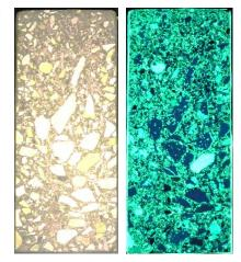
In order to evaluate the consequences in durability, two cores, 100 mm in diameter and 230 mm long, were drilled out. A 50 mm thick slice was cut from the top end of the cores (the cover layer) and conductivity measurements with MERLIN were performed on these slices and compared to measurements of the center part of the cores (bulk concrete).
