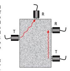
at different times to determine changes of UPV with time. It is also highly repeatable. For tests of sound concrete, the coefficient of variation for repeated measurements at the same location is 2 %. The accuracy of the pulse velocity is a direct function of the accuracy of the measured distance between the transducer faces.
