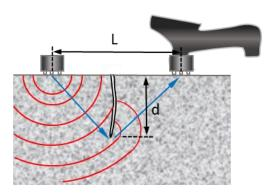
midpoint between the transducers. By using these transit times and the distance between the transducers, the crack depth can be calculated:
