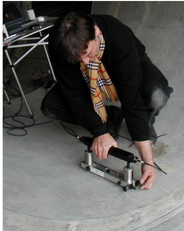
Measurement of P-wave speed by surface method
