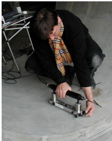
Measurement of P-wave speed by surface method
