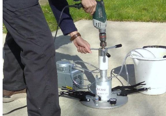
The CS-75 coring rig attached to the suction plate before conducting BOND-TEST
