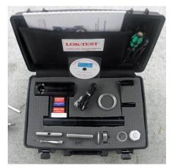
The pull machine can be used for pullout test (LOK and CAPO tests)
