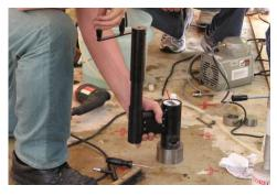
The procedure and special equipment used for the **BOND-TEST** ensure that the disc is loaded in direct tension without bending. Bending may lower results by 20 to 50 %. The discs have sufficient stiffness to avoid distortion during testing. By bonding a clean disc on a planed, dry surface with the GRA adhesive, failure should not occur at the disc/overlay interface. Failure at the disc/overlay interface is an inconclusive test and must be repeated if the bond strength is to be evaluated.
