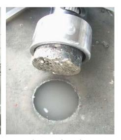
BOND-TEST being performed for quality control of the bond between a wear resistant overlay and a concrete slab; coring after bonding the 75- mm disc is shown (left), application of pull-off load (middle), and the bond failure, type (b), between the overlay and the substrate (right) at 1.8 MPa
