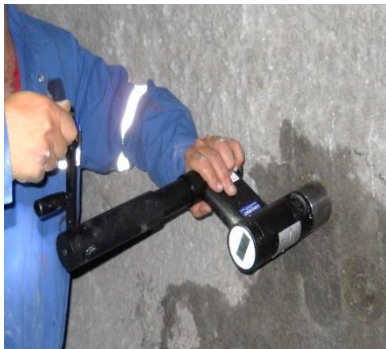
Strength testing of shotcrete, mine shaft, Canada
