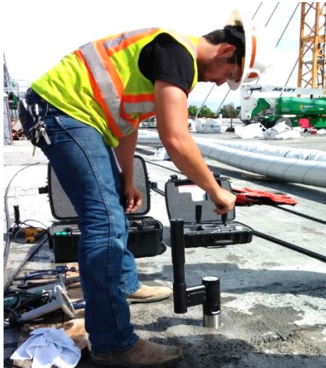
Testing of bridge joint before final loading, USA. Adjacent, the CAPO pullout cone
