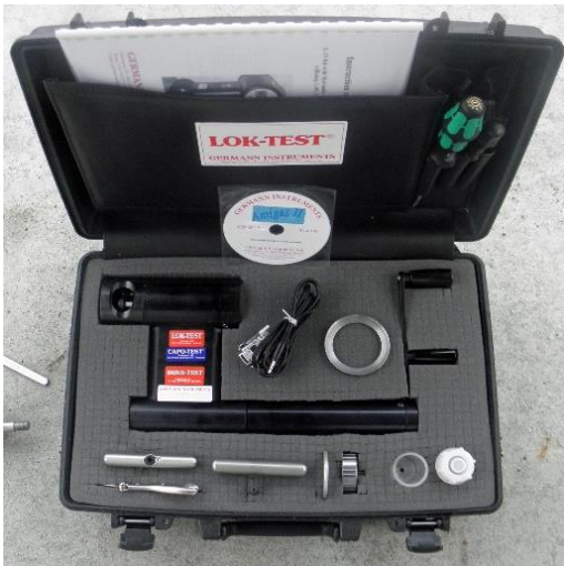
The L-11-1 pull machine can be also used for CAPO-TEST and BOND-TEST . See their Technical Data Sheets.
