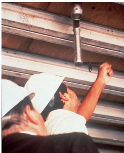
LOK-TEST being performed on a wall for quality control of the finished structure. “H” on the display shows the highest pullout force. The L-40 Insert is used.
