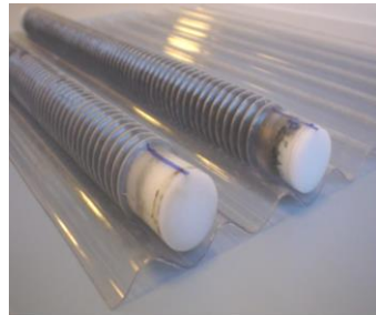
Place the tubes on a grooved rack until setting
