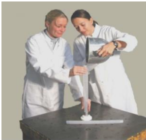
Fill the corrugated tube and install end-plugs
