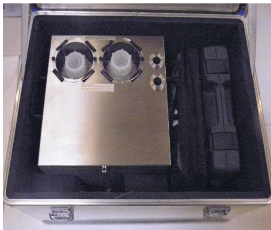
Aluminum case with water tank for de-aerating and tempering, laptop and drill machine
