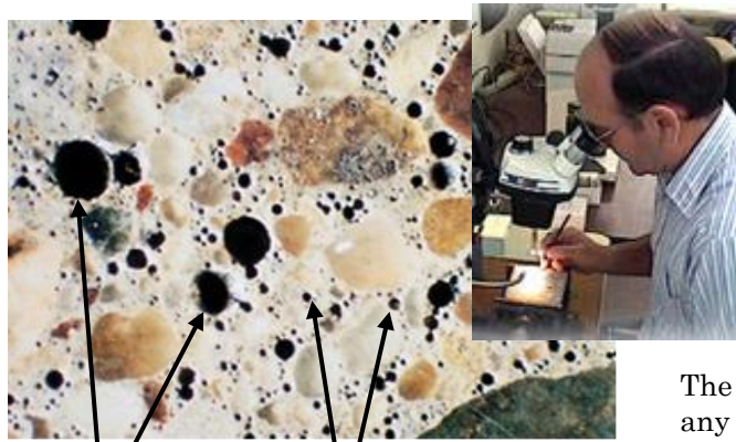
Entrapped air bubbles >3 mm diameter Entrained air bubbles <3 mm diameter (2 mm cord size)
