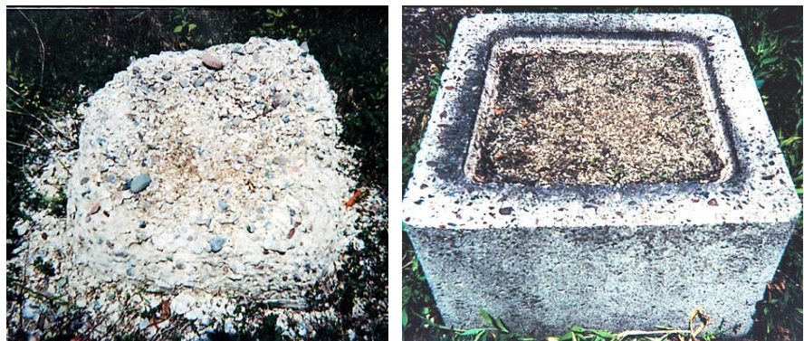
Example of outdoor exposure to Freezing and Thawing after 40 years.
